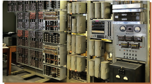
ANTIQUATE HARDWARE. A vacuum type computer named as Harwell Dekatron made in 1951. Photo from www.flickr.com
